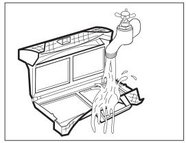
**6.** If necessary remove fluff from the filter socket and gasket. You can use a vacuum cleaner. Put the filter inside the filter socket.
