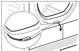
**3.** Turn 2 blockages to unlock the condenser cover.
