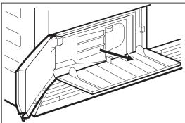
**6.** Clean the condenser in vertical position over a basin or paddling. Rinse through with a hand shower.
