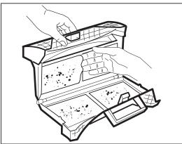
**5.** If necessary clean the filter with the brush under warm tap water and/or a vacuum cleaner. Close the filter.
