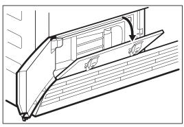
**5.** Catch the handle and pull the condenser out from the bottom compartment. Move condenser horizontally to do not spill remaining water.
